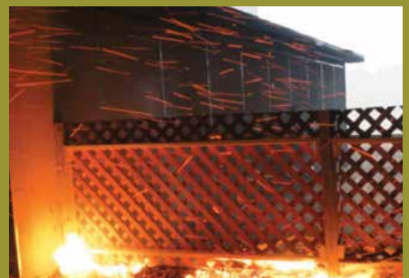
Flame spread to the building when combustible debris was at the base of the fence.
